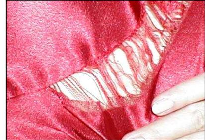
If you are sewing homogeneous type fabrics like leather or vinyl, you will not usually have “seam slippage” but the fabric rupturing under extreme stress.
