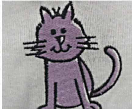
**DESCRIPTION:** Where the stitches and design elements do not line up correctly. The embroidery sewing process sews different colors at different times. If the fabric shifts while one color is being sewn, then poor registration will occur when the next color is sewn. Sometimes it is difficult to tell the difference between poor registration, poor digitizing, and fabric “grin-through” or “gapping” due to thread “pull”.
