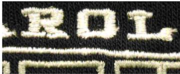
**DESCRIPTION:** Where the corners of lettering or shapes are not sharp and crisp but are bunched up or distorted. Usually caused by too much thread in the corners due to poor digitizing. This includes: 1) Not using appropriate stitch selection, 2) Not using “Short” stitches in corner, and 3) Poor stitch balance – thread too loose..
